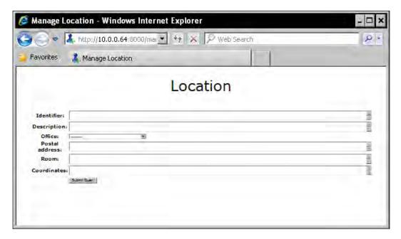
And we specify a text-align of right, instead of center, for the th elements Django ModelForm uses for labels. A text-align of left would also be an improvement, but not quite the same:
