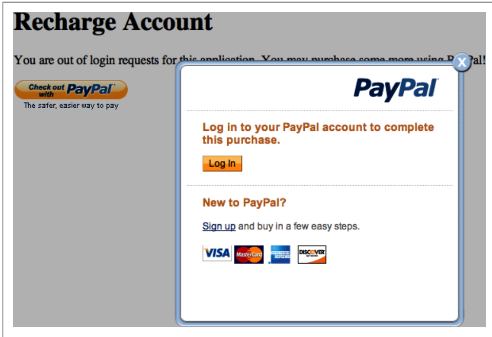
Figure 3-2. When the user clicks the PayPal button, an inline frame is spawned in the page. When the user clicks the Log In button, it spawns a new browser window that is used to initiate the login process. (See Steps 1–4 of Figure 3-1.)
